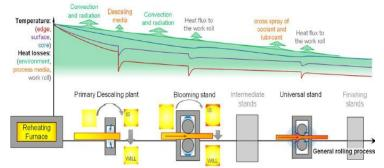
Overview of heat losses along the rolling process of long products
